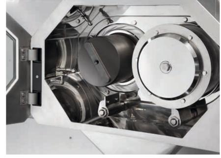
The BRC can be dismantled with just a few turns, ensuring a quick cleaning.
