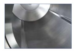
the exhaust air plenum. Thus process air as well as atomized suspension flow in parallel. Process air flows directly through the tablet bed from the inlet air plenum into the outlet air plenum. The portion which leaves the tablet bed into the coating pan is pulled in laminar flow, without turbu-
