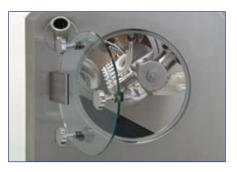
vidual return flow assembly for recirculation of the suspension flow. This feature allows the coating suspension to stay in flow during the beginning or towards the end of the continuous process to avoid sedimentation during spray interruptions. Each nozzle group can be controlled individually to precisely adjust the required spray rate.
