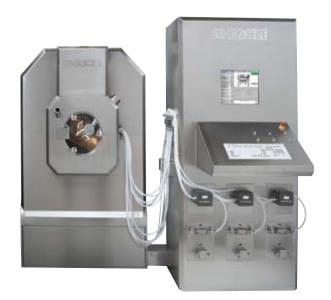
grated discharge module which is individually driven to control continuous discharge. To constantly measure the gun to bed distance, a laser measurement system is integrated into the spray arm. The measured value is used to determine and maintain
