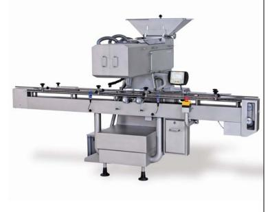
**CF-1220:** 12-channel high-speed tablet and capsule counter with single-track bottle conveyor.
