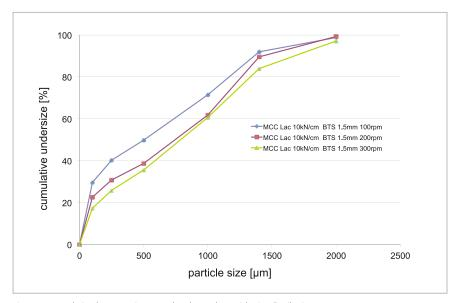
Figure 5: Interrelation between sieve speed and granule particle size distribution
