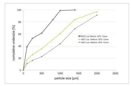
Figure 2: Compaction force impact on granule particle size
