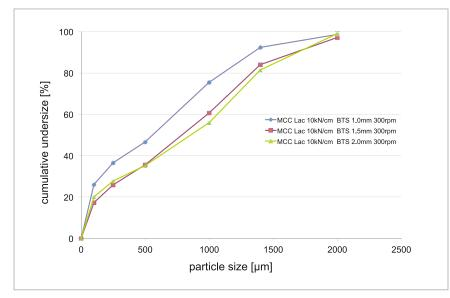
Figure 4: Impact of screen size on granule particle size distribution
