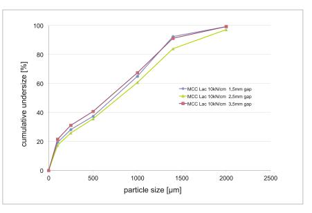
Figure 3: Influence of gap width on granule particle size
