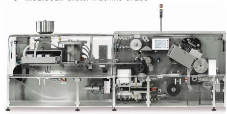
The **CP200** is a highly compact blister machine with a very small footprint and a capacity of up to 250 blisters per minute. The extremely short change-over time makes this machine ideal for the efficient packing of small lots as well as clinical trials. A direct transfer to a MediSeal cartoner is possible.
