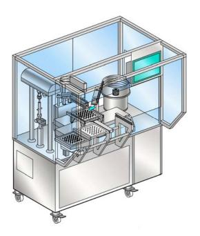
**DFVN 1000 EM**: Filling and stoppering machine for presterilized disposable syringes in the nest.
