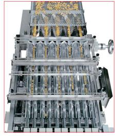
Precise guidings and adjustable flap rows feed the tablets fast and troublefree through the sorting channels in single file.
