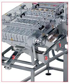
Removable discharge channels for (1) too thin, (2) good and (3) too thick tablets on Seidenader sorting machine. Open design, easy to clean.
